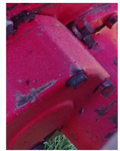
locations for two bolts that would come out while the third hole provided the position of the sheared bolt.
