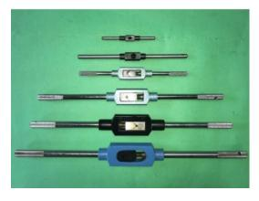
bars to provide access and then a 'T' bar to turn the tap. A ratchet or any type of offset bar isn't a good idea as off-centre forces will tend to push the tap off centre and greatly increase the risk of a damaged thread and/or broken tap.
